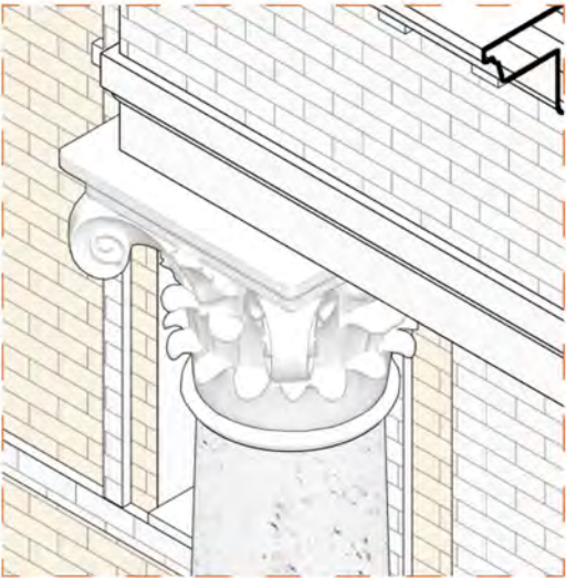
Reconstruction of the column capital in white stucco
